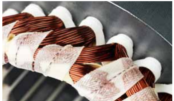
The coil ends are always manufactured within the dimensional tolerances.
